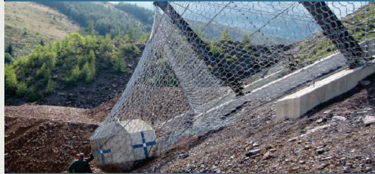
A completed Maximum Energy Level test for a 5000 kJ rockfall catchment fence.
