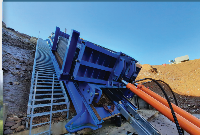
This inclined test facility is one of the largest and most modern in the world. It can accommodate a large variety of types of fences as well as earth dams.
