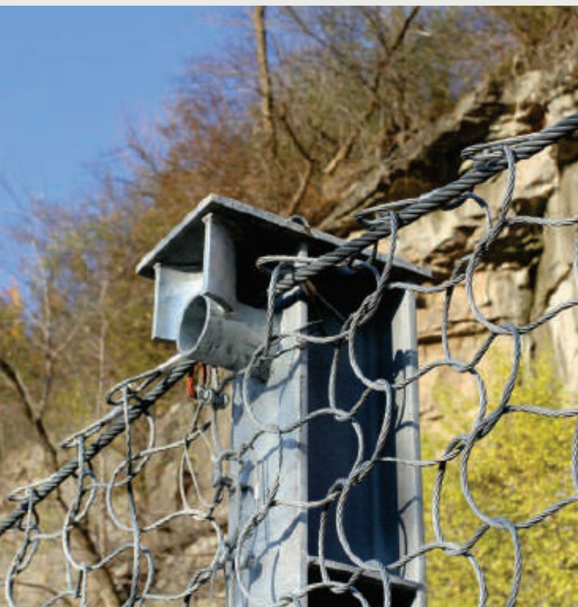
The rope guidances on the posts and base plates are integrated and designed to be robust, giving the ropes smooth surfaces to glide over during an impact to help minimize fatigue. There is no assembling required.
