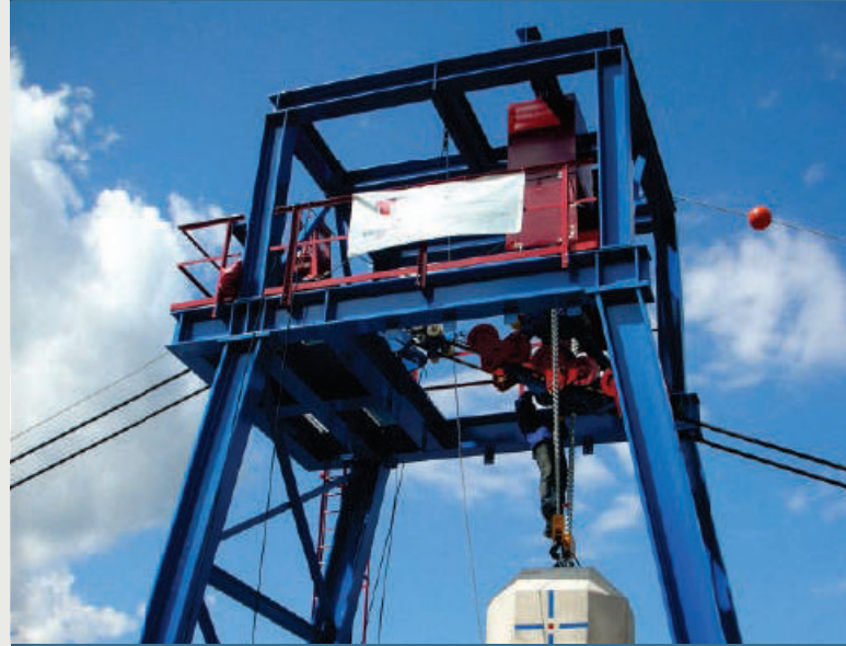
Tests following certification guidelines are carried out using standardized blocks to simulate impacts up to more than 5000 kJ.
